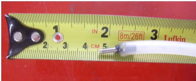
Figure 3.16 Pitot and Tygon® tube connection.
