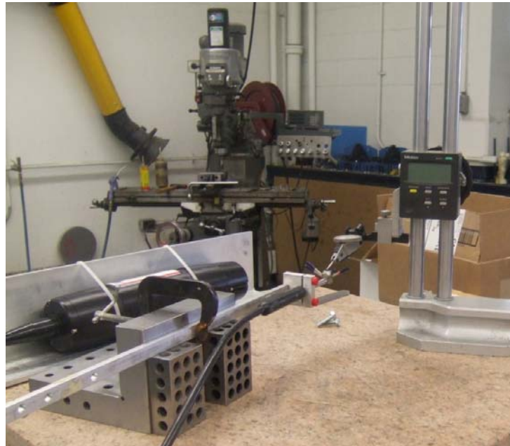
Figure 3.11 probe face alignment, broad view
