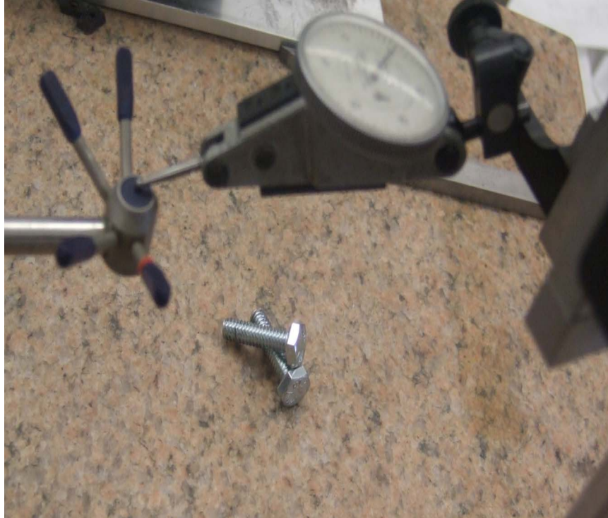
Figure 3.12: probe face alignment. If the needle on the gauge remains stationary as the probe face is moved, the entire face is level.
